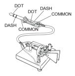
For straight-key operation, only the tip and shaft connections are used.
