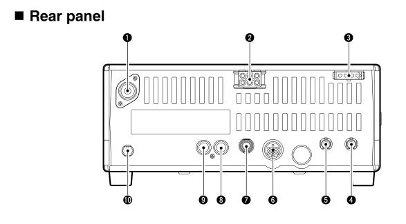
**O ANTENNA TERMINAL [ANT]** (p. 10) Connects a 50 Ω antenna with a PL-259 connector and a 50 Ω coaxial cable.
